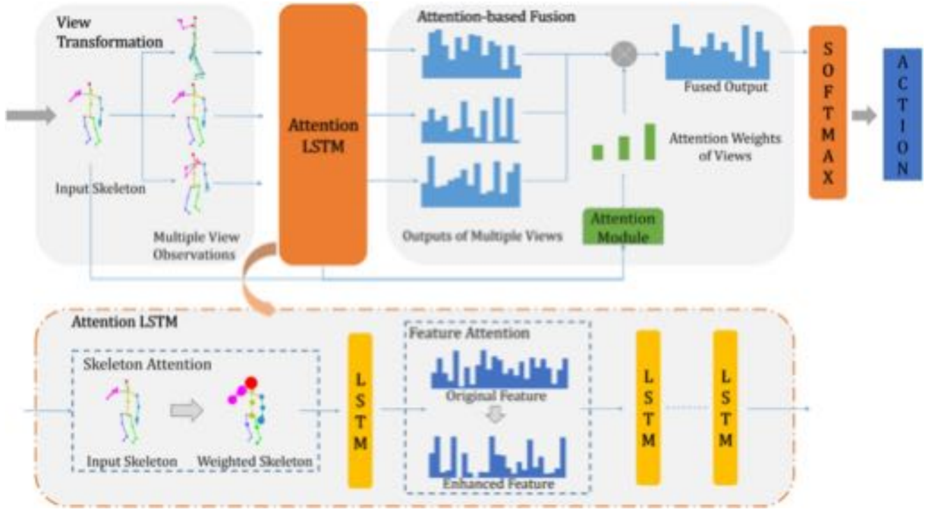
Fig. 1. Framework of our proposed model. There are two essential components in our work. 1) Attention-based multiview re-observation fusion network, which forms the overall framework of our model. The input skeleton is first transformed into several possible view observations. These skeleton observations are processed by the proposed attention LSTM separately, and their outputs are fused for the final result. In the fusion process, an attention module generates weights for different views to highlight the helpful views. 2) Attention LSTM, a multilayer LSTM network integrated with attention. In attention LSTM, the input of every LSTM layer is enhanced with feature attention.
